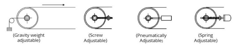
NOTE: Ensure that belt take-up adjustment is the same on each side of the conveyor.
