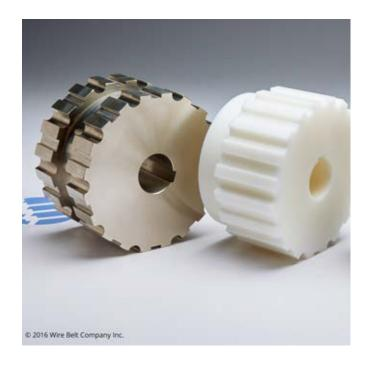
With their positive engagement, sprockets eliminate the possibility of slippage on the drive shaft that can occur on a friction drive system. All sprockets are available in stainless steel or polyacetal plastic. The table below shows the available pitch diameters and number of teeth for each belt pitch.
